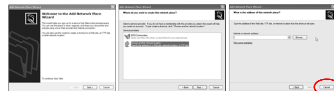
(a) Add Network Place wizard. (b) Select a service provider. (c) Address of the network place.
